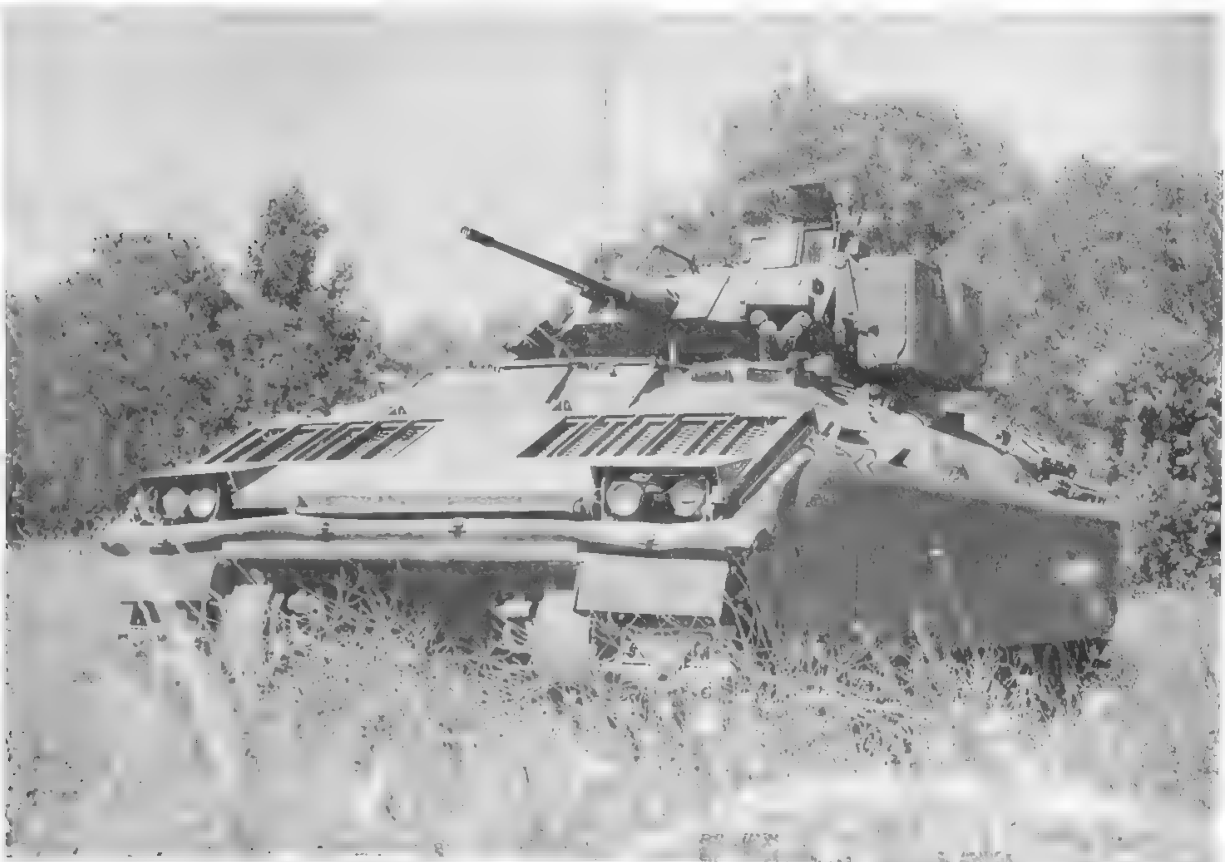
While the M2 Bradley resembles a late production M113, it is a much larger and heavier vehicle. The trim vane fitted to early model vehicles can be seen here. (U.S. Army photo)
